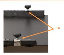
3. Rotate the screws clockwise to clamp the base plate onto the couch edge. Make sure the screw is located into the foreseen hole in the base plate. There is no need for a high clamping force so fix manually with light strength. Overdoing the clamping force may damage the couch!
